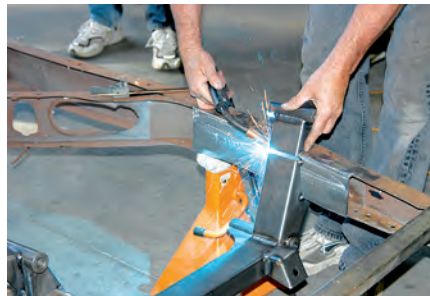
12) After the towers lined up perfectly, they were tack-welded to the frame. All of the measurements were made again to be certain they were correct. When O'Bryant was satisfied, the towers and crossmember were finish-welded to the frame.
