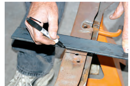
5) The HEIDTS® centerline was drawn on top of the frame to make it easy to spot.
