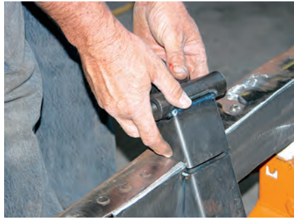
11) The upper A-arm mount or tower had to be installed next. It was placed on the frame and extends upward from the lower crossmember.
