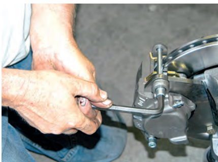
22) After the rotor was installed, O'Bryant tightened the Allen bolts with a 3/8-inch Allen wrench. At this time, you should make sure that the rotors are centered between the calipers.
