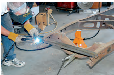
1) A heavy-wall-thickness square tube was tack-welded to the chassis to hold it in place when the stock crossmember is removed.
