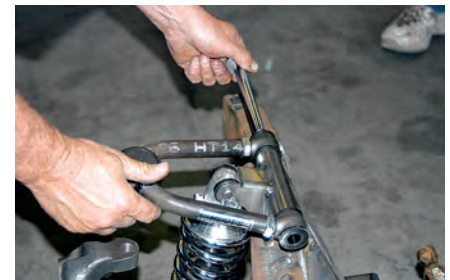
18) Using the other long bolt supplied in the kit, the upper A-arm was installed. This connection also uses the large washers supplied in the kit. The upper bolt is secured with a Nylok locknut.
