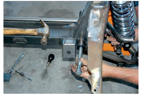
15) The lower A-arm was installed using the long bolt supplied in the kit. Washers are supplied to rest against the urethane bushings.
