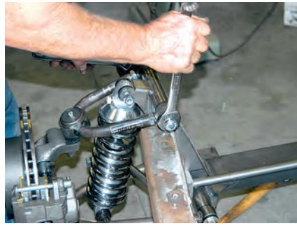
23) After all the front suspension parts are installed, the bolts can be tightened. The upper A-arm bolts were secured with a pair of 15/16-inch wrenches.
