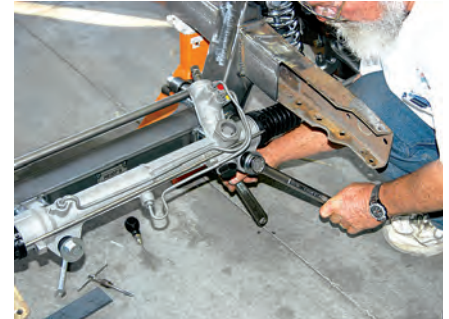
26) The rack-and-pinion unit was reinstalled and then it was tightened with a pair of 15/16-inch wrenches.
