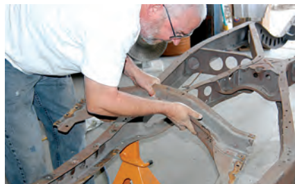
3) The crossmember was easy to remove when it was moved back to the wider part of the frame. Since these crossmembers are worth money to nostalgia rodders, owner Bob O'Bryant wanted to keep it in good condition. The radiator mounts are still attached to the crossmember and will have to be removed and used after the new front suspension is installed.
